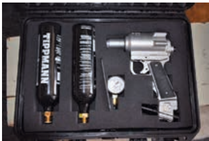
Non-penetrating captive bolt gun acceptable for humane euthanasia of piglets under 9 kg.
